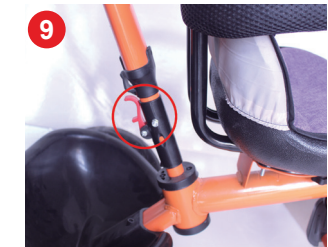
9 Rotate the red lock inside the ring to lock it
