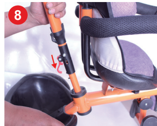
8 Place the handle of the tricycle in the rear axle and adjust the direction
