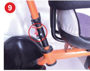
9 Turn the rear wrench inside the ring to lock it up
