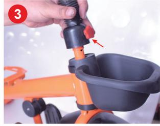
3 Put the front handle into the front basket and align the screw holes to tighten the screw cap
