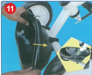
11 Install the rear basket and firmly pull the storage basket into the corresponding position as shown in the figure
