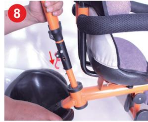
8 Push the back pusher into the rear steering lever and align the direction
