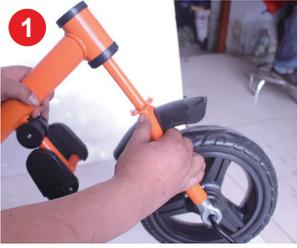
1 Install the front and the front forks into the head tube of the body
