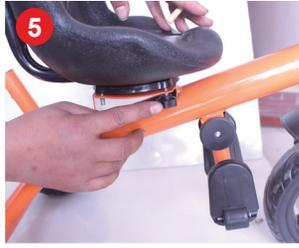
5 Install the seat, insert the seat screw into corresponding screw hole, and fix it with the black knob.
