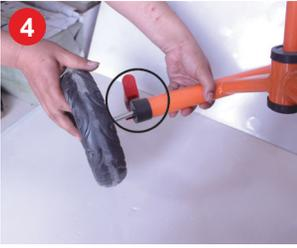
4 First install the brakes on the frame slot, then insert the rear wheel into the clamp
