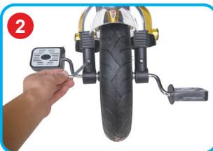
Insert the front wheel into the front fork and fasten it with screws and tighten it.
