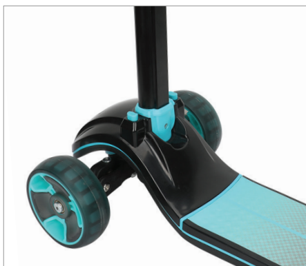
③ The pole is inserted, and make sure the marbles pop up.
