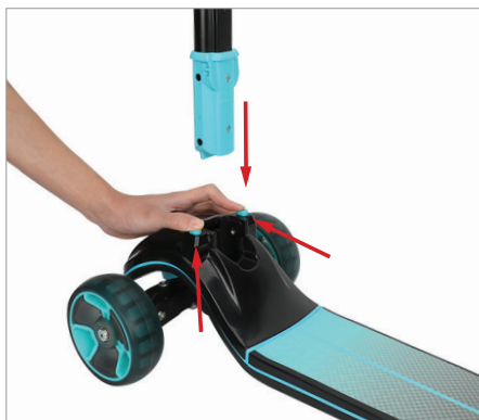
② Press down the 2 buttons on the front of the scooter, then insert the rod.
